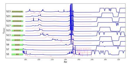
Relaminarisation times for EQ (blue) and TW (red) saddle-node states. Midplane of streamwise velocity of EQ saddle-node states is shown on the left.
